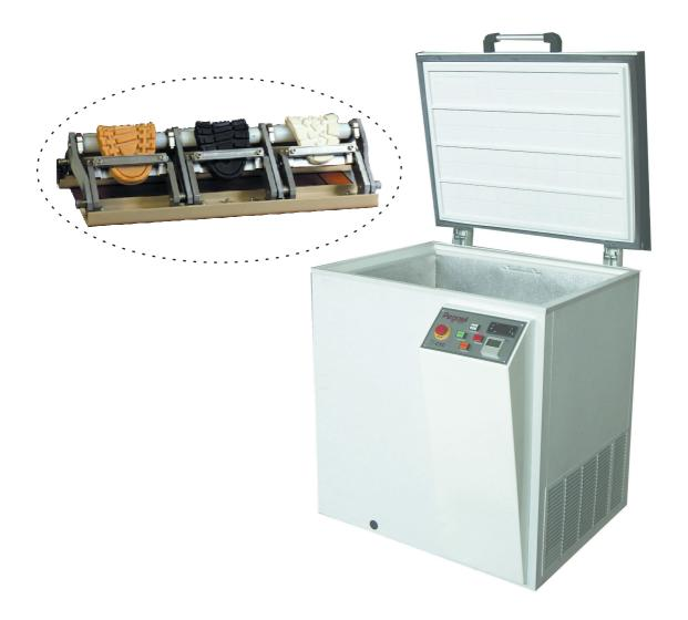
"BENNEWART" flexing machine with cold chamber
